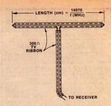
For use indoors, this dipole can be made up from a length of ordinary 300-ohm antenna twin-head, either black or opaque. The joints could be twisted but soldering provides a more reliable connection.
