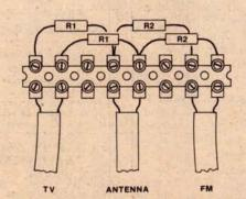
Shown above is a simple way of making a 2-way splitter for a 300-ohm TV antenna down-lead. The arrangement of the isolating resistors varies from this in some of the commercial splitters but, presumably, they would do the same job.
